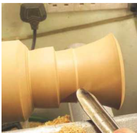
▲ Pic.13 Once you are happy with the inside shape you can start to remove the excess wood from the outside, keeping the bevel of the tool in contact and working it down in stages
